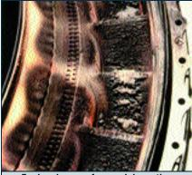
Engine damage from ash ingestion
